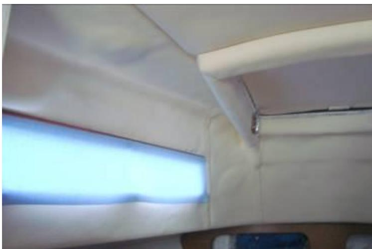
For that part lying under the mast, the lining was glued to a sheet of hardboard which was screwed in place – this allowed access to mast foot bolts. The rim of the hatch was covered using separate strips of headlining but using the overlap technique described earlier where there were butted joins.
